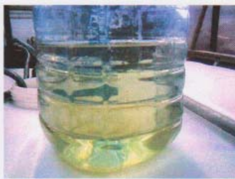
Washing water, cleaned and without mechanical impurities and coagulate
